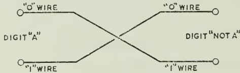
FIG. 10/4. Logical element Not or Complement of
